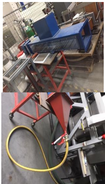
Figure 6. Chamber connected to the air control panel.
